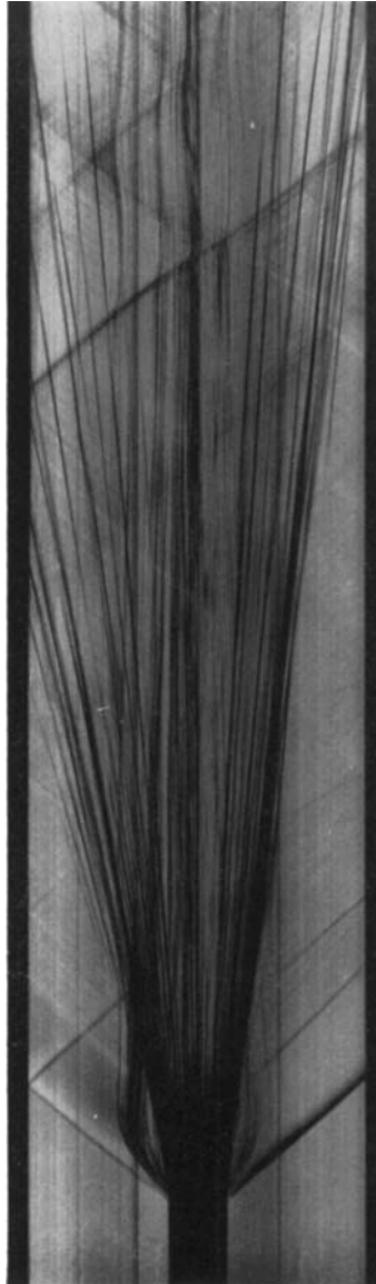
FIGURE 12. Schlieren (r, t) -plane record of the explosion of a 2 in. diameter sphere of helium initially at 326 p.s.i. Shock reflexion from an SLM pressure gauge appears on the left. p_1 = 14.5 p.s.i. T_{1,4} = 25.5^\circ\text{C} .
